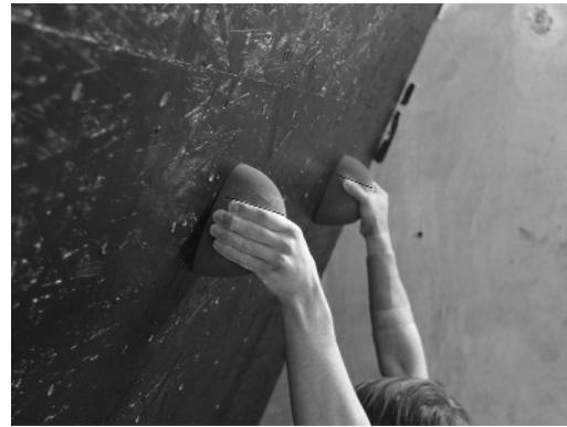
Figure 4. Nr. 01 pinch grip (Skyroof) with the thumb opposed to the fingers. The optical markers (black lines) guarantee a standardized gripping.
